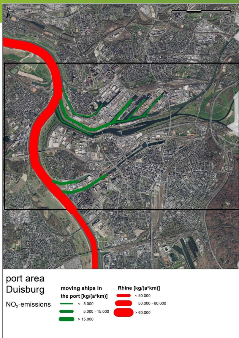
Figure 15: Representation of the emissions calculated according to the new method from ships sailing on the Rhine and in the port in the study area of Duisburg as line sources.
