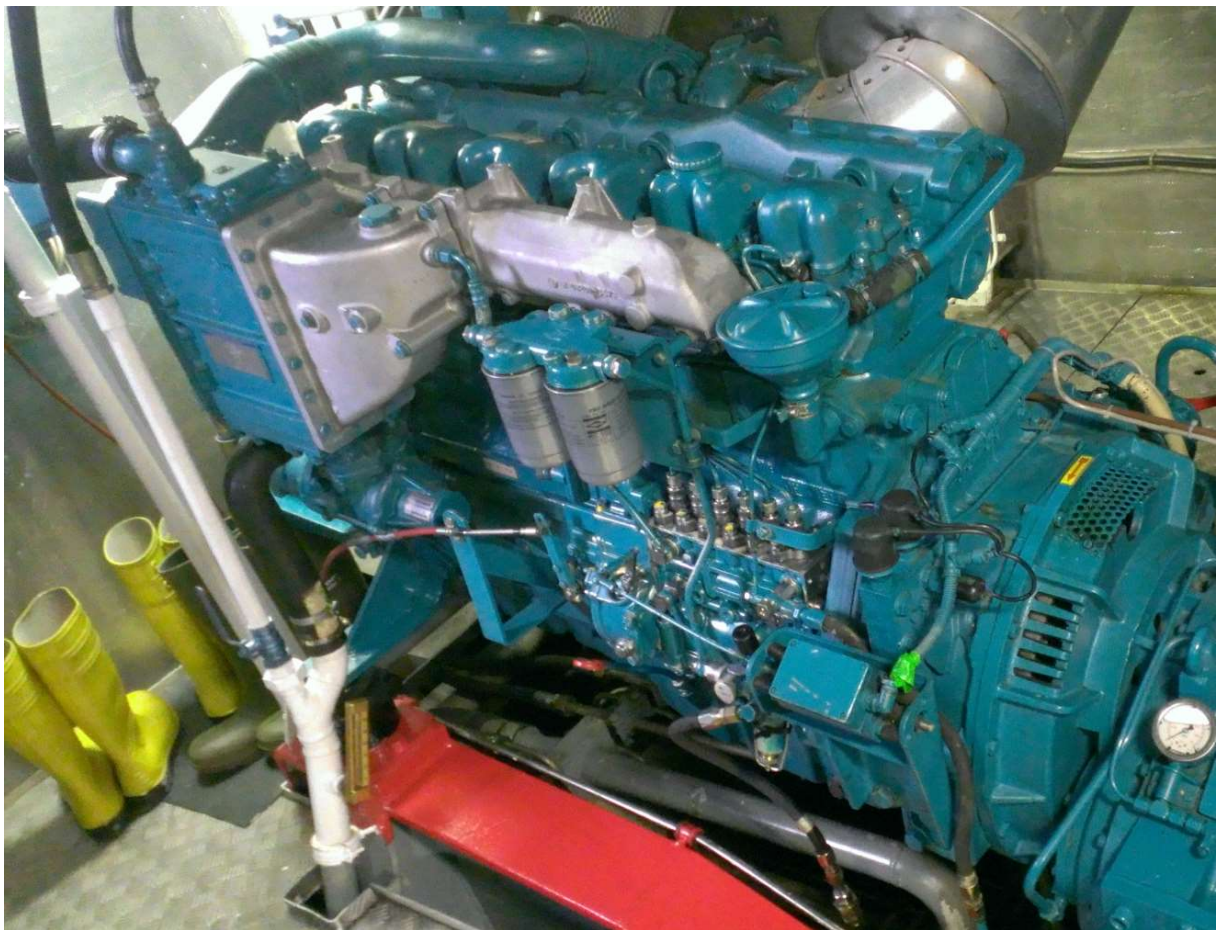
Figure 2: Starboard propulsion engine MAN D2866 LXE43
