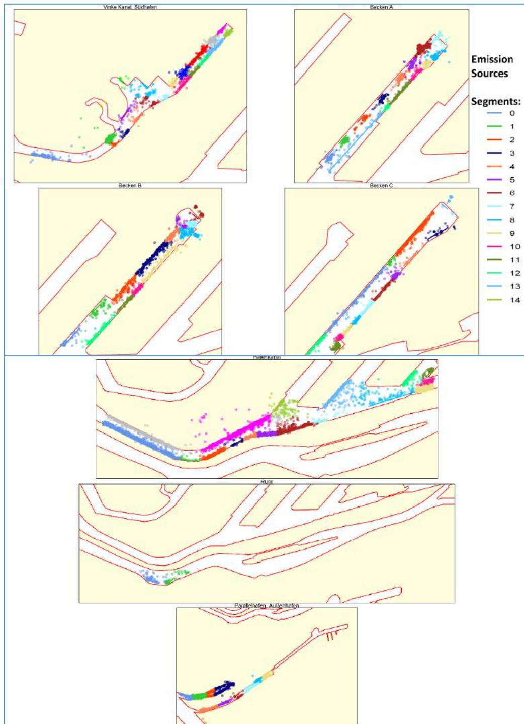
**Figure 8:** Allocation of the point data of the individual ships to the respective line sources (Port of Duisburg).
