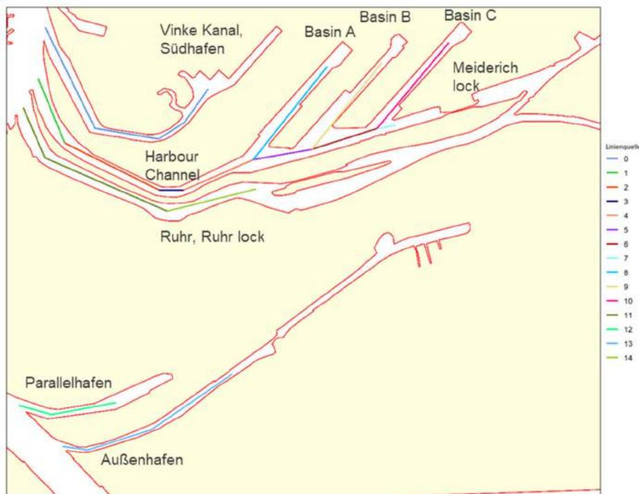
**Figure 3:** Segments of NO<sub>x</sub> line sources for ships sailing in the port of Duisburg
