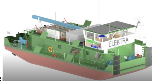
First push boat with Hydrogen Fuel Cell (D)
