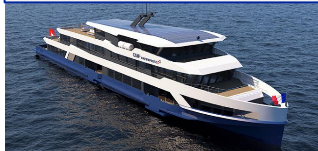
Passenger ferry CNG-electric (CH)
