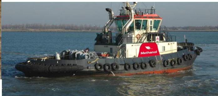
First vessel with exchangeable ZES battery containers for propulsion (NL)
