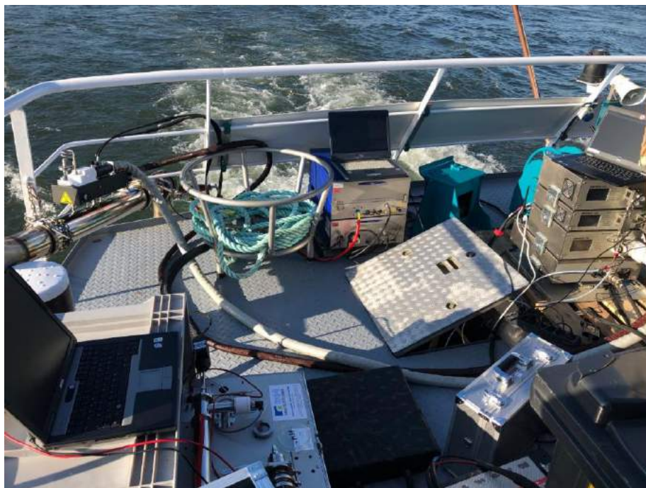
Figure 14: System Arrangement for Measurement downstream AGN ("End of Pipe" (Gaseous, Particle / Soot and Exhaust Gas Mass Flow))
