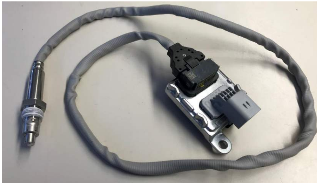
Figure 31: NO x -Sensor [Source: TÜV-Nord]
